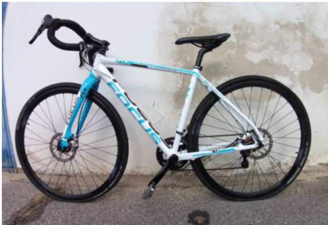
cx FOCUS AX (Al) tg S trasmissione Shimano Deore, freni a disco meccanici Avid cerchi Concept, gommata Schwalbe Racin Ralph
